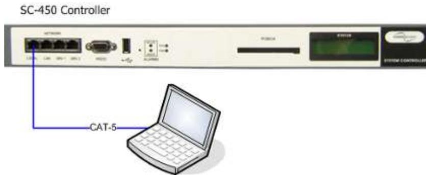
Figure 3-1: Ethernet Cable Connection
