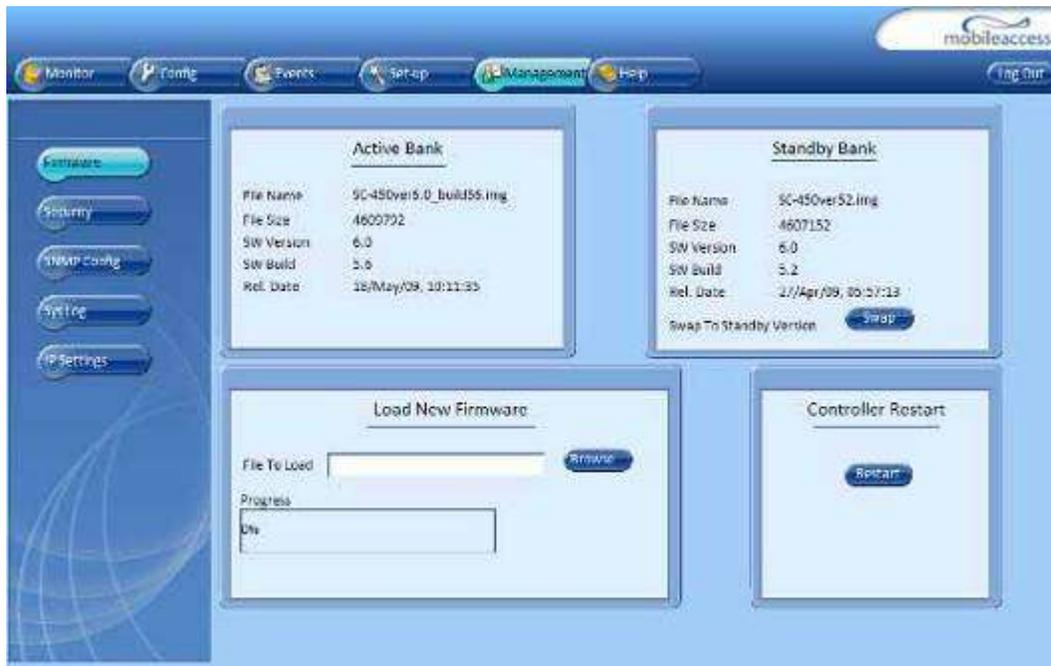
Figure 8-11: Restart System Controller Window
