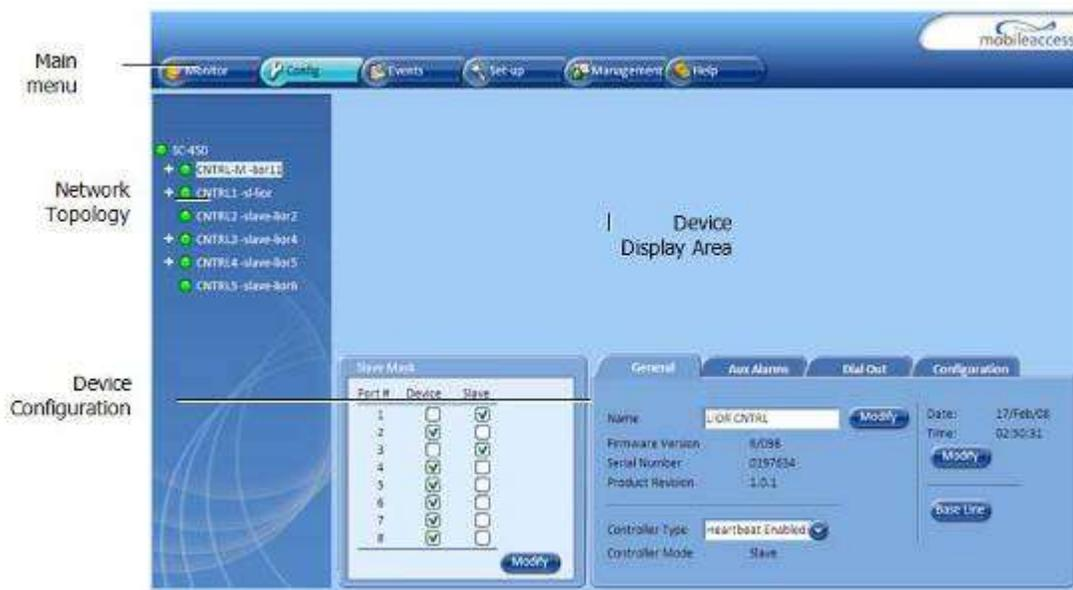
Figure 5-1. Web GUI Configuration window
