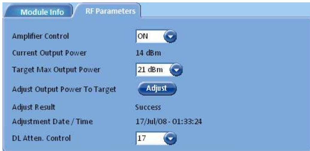
Figure 5-24: Addon RF Parameters Tab
