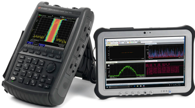
Figure 10. Through a LAN connection, an APCO-25 two-way radio signal is fed into the 89600 VSA Software for detailed analysis.
