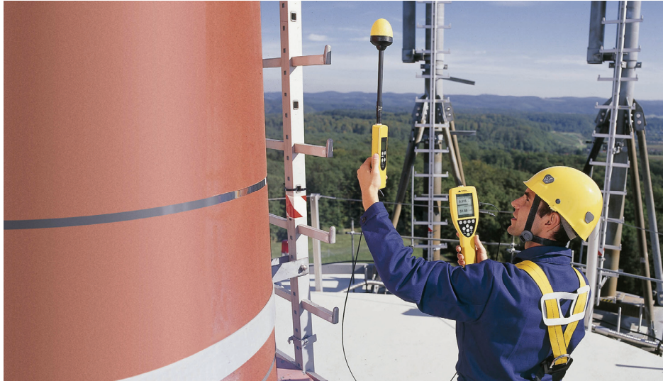
Figure 3. The NBM-550 radiation meter represents the latest generation of broadband instruments and incorporates spatial as well as time averaging, the ability to export measurement results to Excel or other spreadsheets, and can be fitted with a GPS receiver that verifies where each measurement was made.
