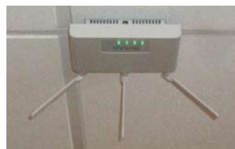
Figure 6. Indoor BelAir 20 mounted on ceiling.
