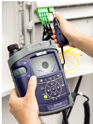
FIGURE 4: SmartClass fiber system with integrated power meter and patchcord microscope
