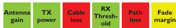
Figure 1 Overview on how to calculate link budget. Items shown in green are added while items shown in red are subtracted. The resultant number is the link budget. The fade margin is recommended to be an extra 20 dBm to account for unforeseen interference.
