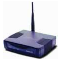
EnGenius 802.11 b/g 400 mW Access Point TESSCO # 330162
