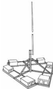
8", 4.5" OD Non-penetrating Rooftop Tripod TESSCO # 488600
