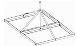
Rohn 60", 1-1/4" OD Non-penetrating roof mount TESSCO # 55966
