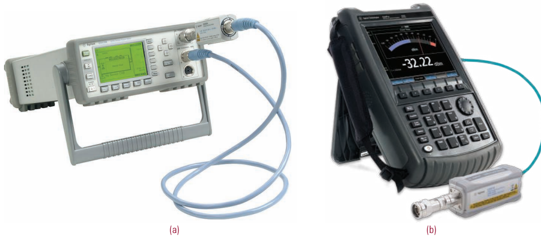
Figure 4. Equipment configurations for measuring RF power using a power sensor with the (a) power meter and (b) FieldFox
